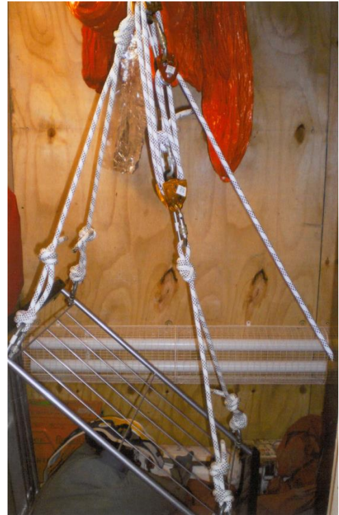
A rig for a nylon stretcher or slick (UK term) - converts from vertical to horizontal without having to rehang it.
