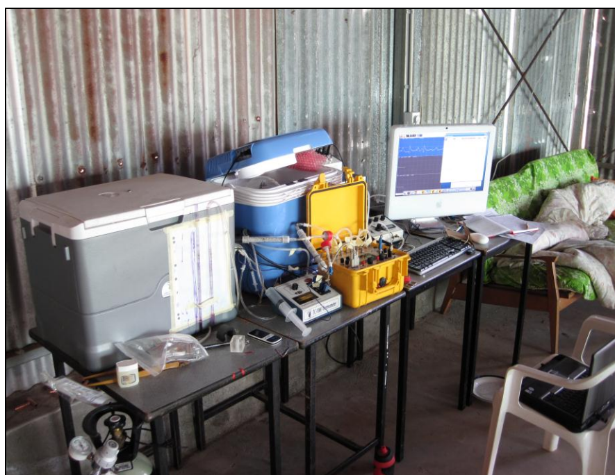
The respirometry equipment set up in the old school house
