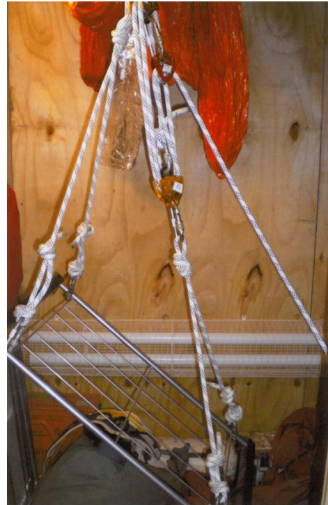
A rig for a nylon stretcher or slick (UK term) - converts from vertical to horizontal without having to rehang it.
